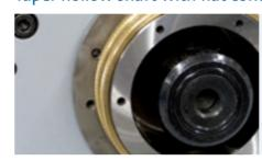
Taper hollow shafts (HSK) with flat contact faces are standardized per DIN 69893-1. The various shapes differ with respect to drive key slots and contact surface. Form C has been especially developed for use with manual tool change systems.
