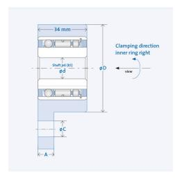
Inner ring clamping direction left available on request. The specified nominal torque refers to the integrated freewheel clutch insert element, not the key way.
