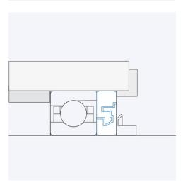
The larger gap diameter  $e_2$  must always face the impact.
