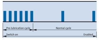
The time duration of the pre-lubrication is dependent on the length of the connected lubricating lines.
